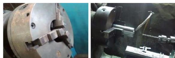
Fig 2: Head Stock of Lathe Before and After Modification
