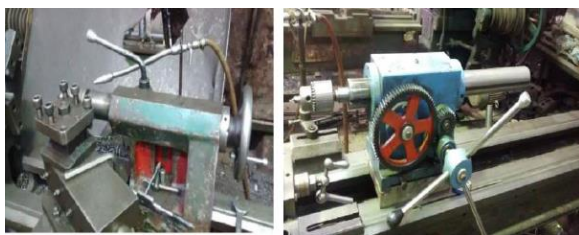
Fig 3: Tail Stock of the Lathe Before and After Modification
